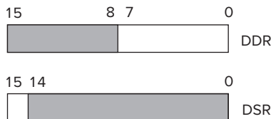
Figure 9.5 Monitor device registers.
