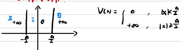
$$\text{定态薛定谔方程化为: } \frac{d^2\psi(x)}{dx^2} - \frac{2m(E-V)}{\hbar^2} \psi(x) = 0$$
