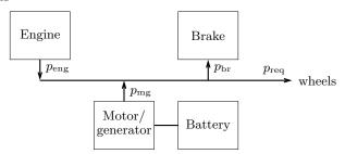
All of these powers are functions of time, which we discretize in one second intervals, with  $t=1,2,\ldots,T$ . The required wheel power  $p_{\text{req}}(1),\ldots,p_{\text{req}}(T)$  is given. (The speed of the vehicle on the track is specified, so together with known road slope information, and known aerodynamic and other losses, the power required at the wheels can be calculated.) Power is conserved, which means we have
