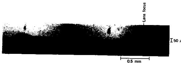
FIGURE 18.15 Damage filament due to self focusing of a Ruby laser beam in sapphire. Sour. Reference 34.
