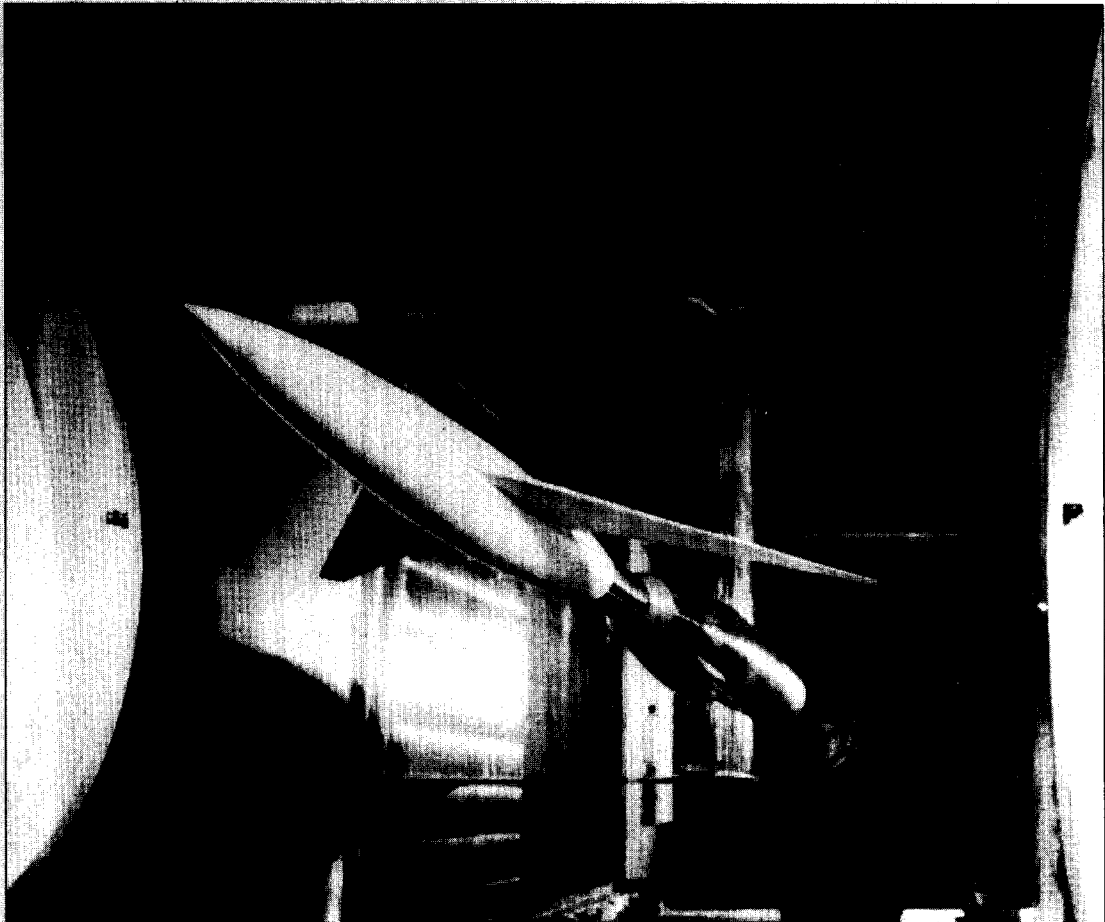
Figure 5.2 | An aircraft model mounted in the test section of the Ames 6 \times 6 -foot supersonic wind tunnel. The test section is labeled as item 2 in Fig. 5.1.
