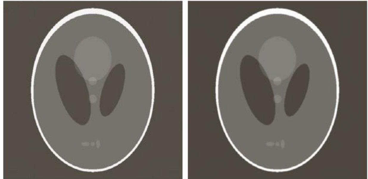
FIGURE 5.44 Filtered backprojections of the head phantom using (a) a ramp filter, and (b) a Hamming-windowed ramp filter. Compare with Fig. 5.40(b).
