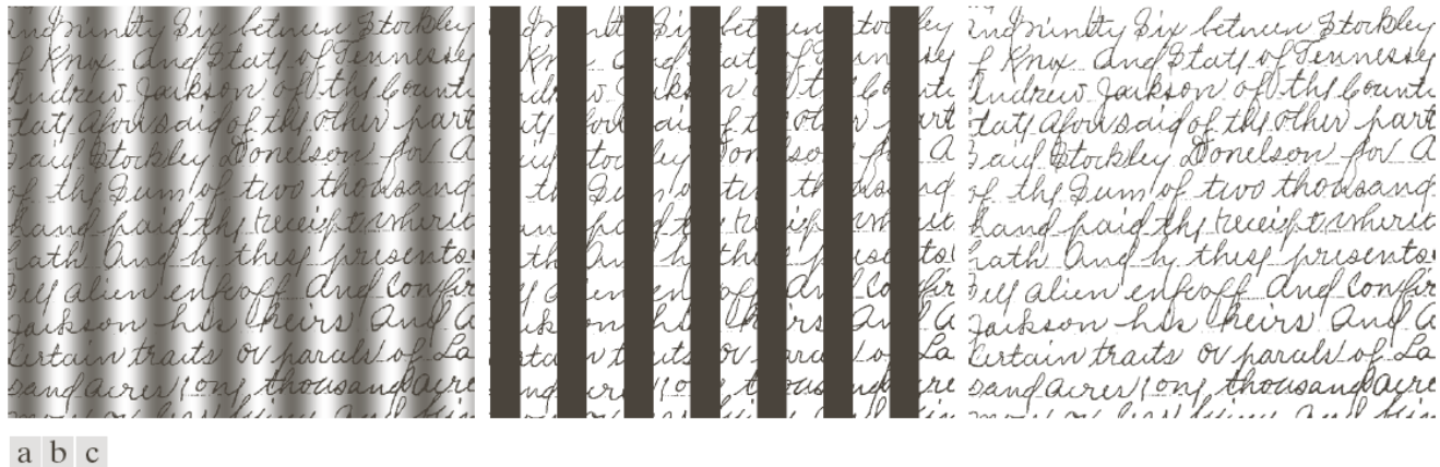
FIGURE 10.50 (a) Text image corrupted by sinusoidal shading. (b) Result of global thresholding using Otsu's method. (c) Result of local thresholding using moving averages.
