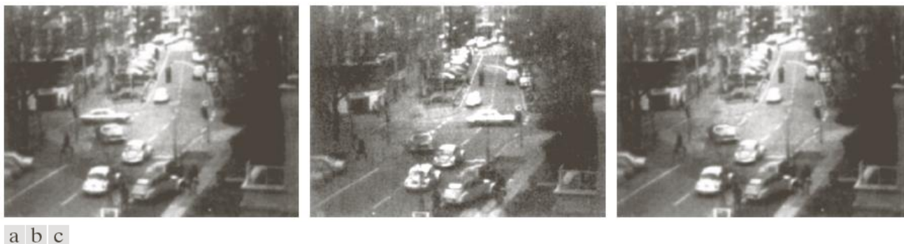
FIGURE 10.60 Building a static reference image. (a) and (b) Two frames in a sequence. (c) Eastbound automobile subtracted from (a) and the background restored from the corresponding area in (b). (Jain and Jain.)
