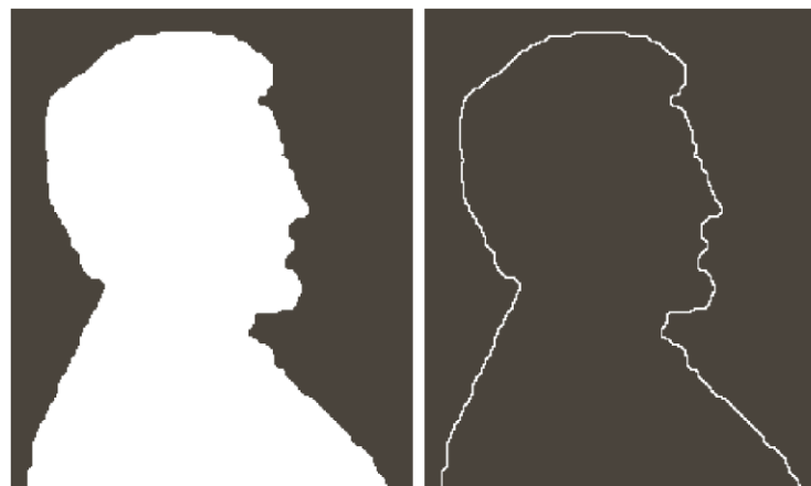
FIGURE 9.14 (a) A simple binary image, with 1s represented in white. (b) Result of using Eq. (9.5-1) with the structuring element in Fig. 9.13(b).
