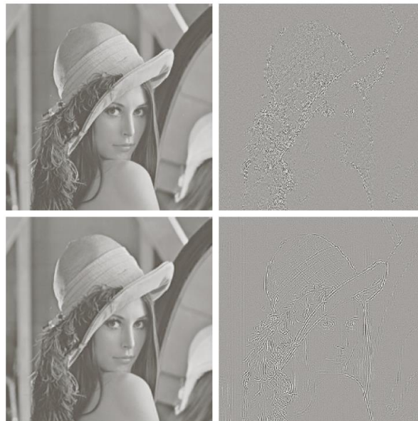
FIGURE 8.28 Approximations of Fig. 8.9(a) using 12.5% of the 8 \times 8 DCT coefficients: (a)–(b) threshold coding results; (c)–(d) zonal coding results. The difference images are scaled by 4.
