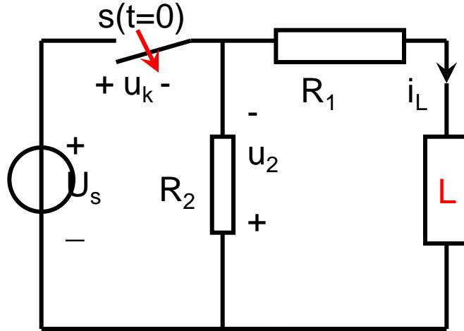
$$U_s = 35V, R_1 = 5 \Omega, R_2 = 5K\Omega, L = 0.4H, t < 0$$
