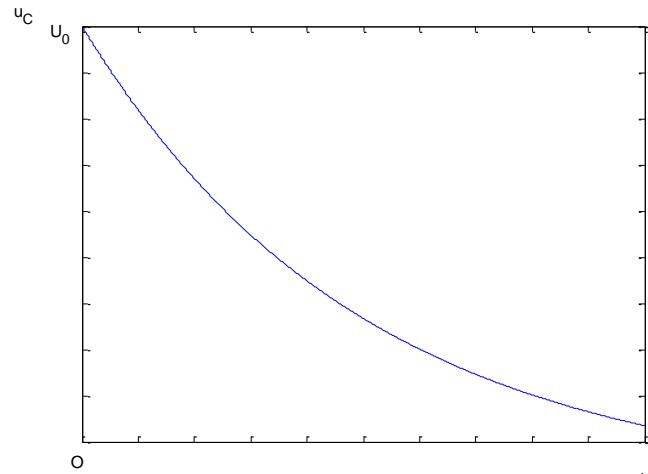
$$\left\{ \begin{array}{l} -u_R + u_C = -Ri_C + u_C = RC \frac{du_C}{dt} + u_C = 0 \end{array} \right.$$
