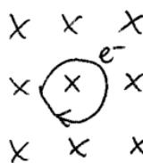
$$\left\{ \begin{array}{l} \frac{mv^2}{R} = evB \\ \frac{1}{2}mv^2 = \mu = \text{Const} \end{array} \right.$$
