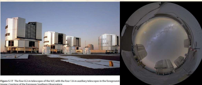
Figure 5.17 The four 8.2-m telescopes of the VLT, with the four 1.8-m auxiliary telescopes in the foreground. Image: Courtesy of the European Southern Observatory.
