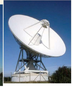
Figure 5.22 The 32-m Cambridge Telescope – a Cassegrain design. The cone houses a carousel supporting four receivers. Image: Ian Morrison.
